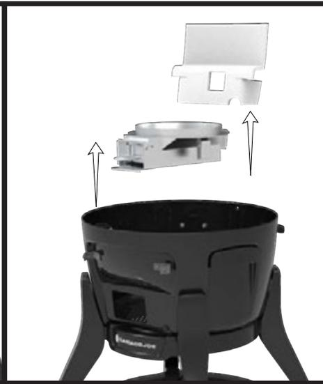
Remove ash drawer assembly and rear insulation. Note - the rear insulation is secured with the ash drawer assembly.
