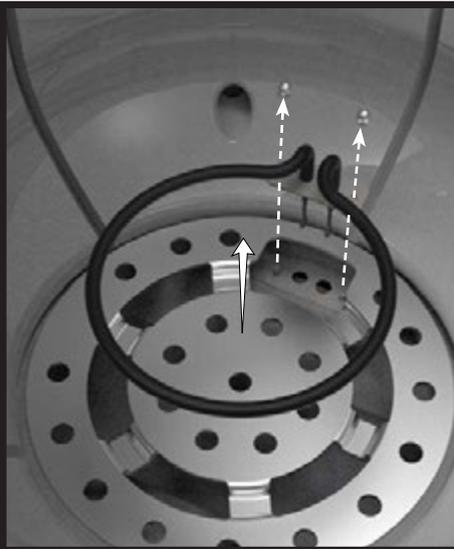
Remove the 2 acorn nuts from the element mounting plate. Then, with extreme caution, lift the element straight up and out of the grill. (NOTE - you may need to lightly hold down the element bracket to remove the element from the bracket).
