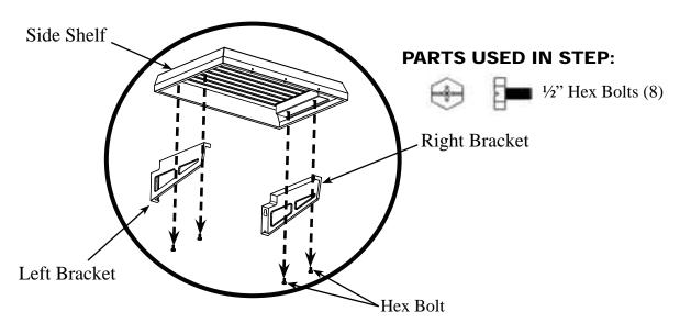
**Step 8** Loosen top two (2)  $\frac{1}{4}$ -20 x  $\frac{1}{2}$ " HEX BOLTS on both sides of GRILL BODY attaching LEFT LEGS and RIGHT LEGS. Attach SIDE SHELVES onto GRILL BODY using four (4)  $\frac{1}{4}$ -20 x  $\frac{1}{2}$ " HEX BOLTS, as shown below.
