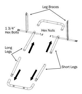
**Step 2:** Install Bottom Wire Shelf by placing the four corner hooks inside the hole on each leg then rotate the leg assemblies up and secure the Leg Braces to the other side of the Long Leg and Short Leg set.
