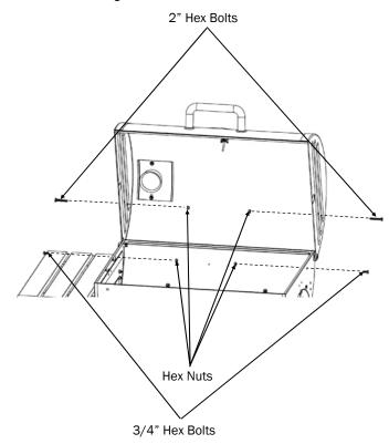
**Step 12:** Place Ash Pan and Ash Pan Hangers onto Grill Body.
