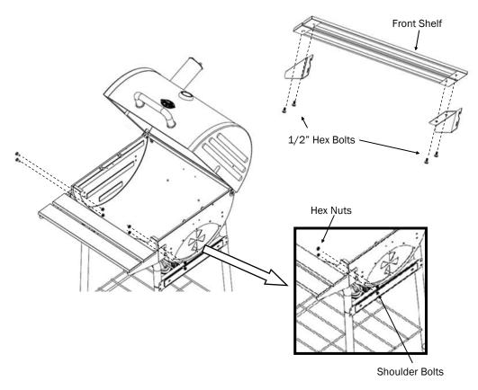
**Step 10:** Attach Side Shelf to Grill Body with four Hex Bolts and four Hex Nuts.
