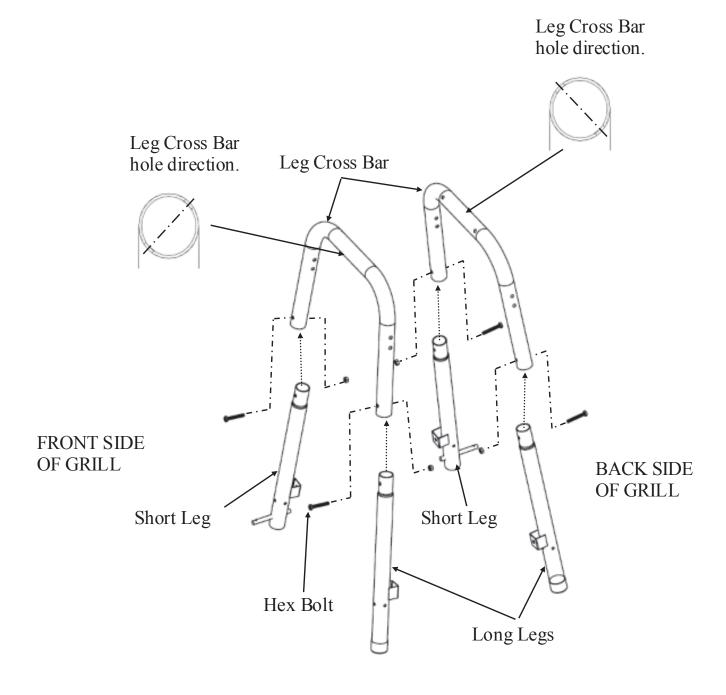
Attach LEG BRACES to the outside of one of the LONG and SHORT LEG and LEG CROSS BAR assemblies from step 1. See below. Use two 1 1/2" hex bolts and nuts for each LEG BRACE but only finger tight.
