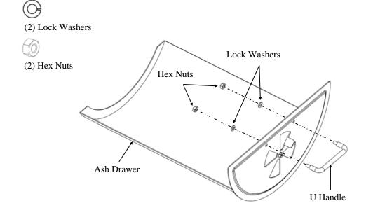
**Step 7:** Tighten ALL BOLTS and NUTS. Insert a 1/2" BOLT and tighten with a NUT for any open holes in Grill BODY after assembly.
