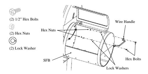
**Step 5:** Attach FRONT HANDLE to SFB HOOD with two 1/2" HEX BOLTS, two LOCK WASHERS, and two HEX NUTS.
