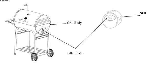
**Step 2:** Attach SFB to main GRILL BODY. With a helper align the SFB in place over the opening on the grill body then attach with six 1/2" BOLTS and NUTS.
