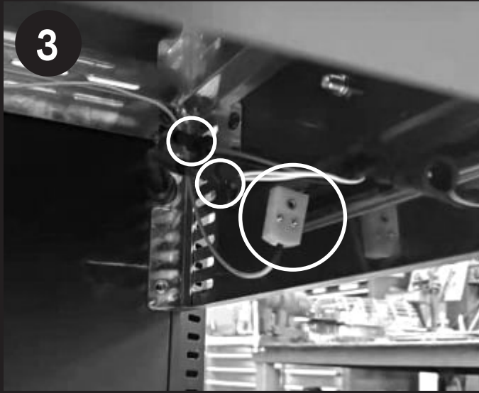
Unplug wires from the controller.
