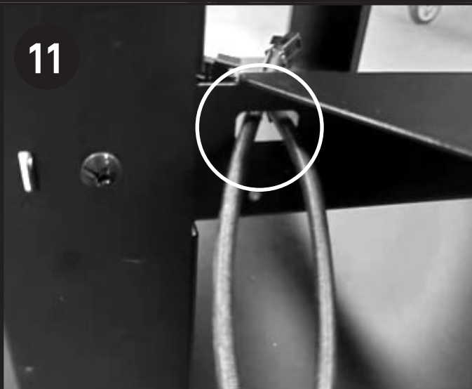
Pull the hopper wires through the leg brace hole.
