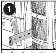
Remove the air intake slide.
