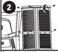
Remove the heat shield by removing the top and bottom screws.
