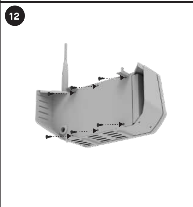
Reinstall the back panel of the controller kit.
