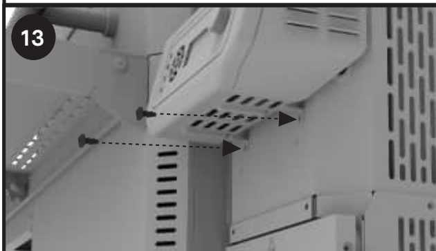
Reinstall the controller kit on the hopper with 2 screws.
