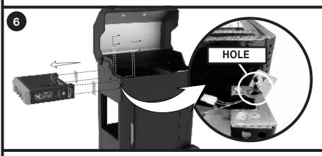
Remove left side shelf. Save for reuse. When you remove the shelf, you have to feed the wire harness wires through the side shelf hole one at a time (white plug and then black plug).
