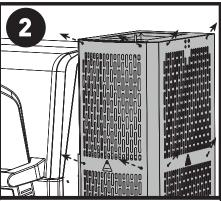
Remove the hopper lid and latch. Remove the heat shield by removing the top and bottom screws
