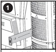
Remove the air intake slides.
