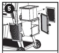
Remove the bottom heat shields and door.
