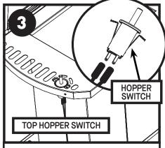
Remove the wiring from the lid switch.
