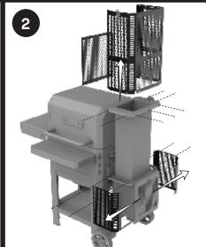
Remove the top and bottom hopper shroud.
