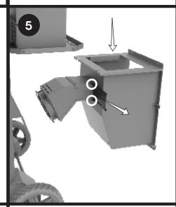
Remove lower hopper and remove the lower slide guide.
