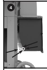
Remove the 2 screws and nuts from lower hopper mounting bracket.
