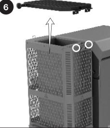
Remove hopper lid (2 screws). Save for reuse.
