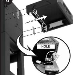
Remove side shelf (4 screws). When you remove the shelf, you have to feed the wire harness wires through the side shelf hole one at a time. Save for reuse.
