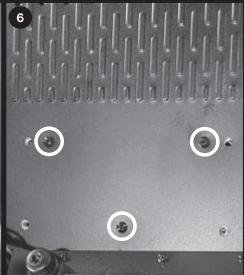
Loosen 3 screws on the insulation housing to make room for the power plug.
