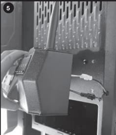
Disconnect two black and white wire connections on the side of the controller.
