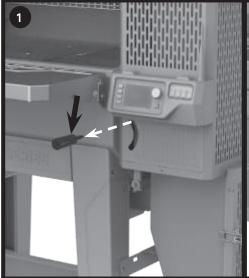
Remove 1 screw on the shutdown flap handle. Unscrew the shutdown flap handle.
