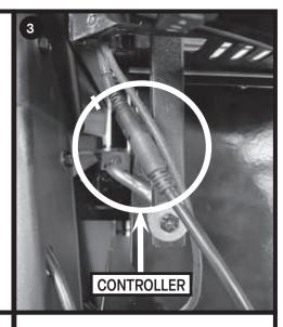
Remove the controller connections.
