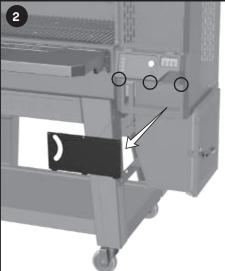
Remove 3 screws on the small hopper shroud. Remove the shroud.
