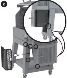
A) Remove the front hopper shroud.
