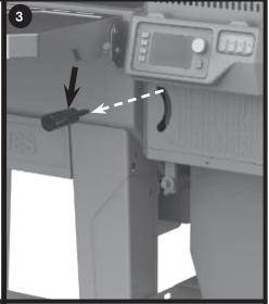
Remove 1 screw on the shutdown flap handle. Unscrew the shutdown slide handle.
