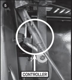
Remove the controller connections.
