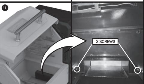
Remove the bottom (2 Screws) next to the manifold inside of the body.
