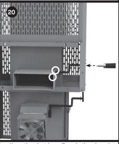
Keep the shutdown flaps in the closed position. Replace the shutdown handle.
