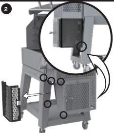
A) Remove the front hopper shroud. B) Remove the hardware that connects the leg brace to the legs.
