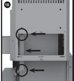
Shutdown flaps and connector rod components should remain in the closed position.
