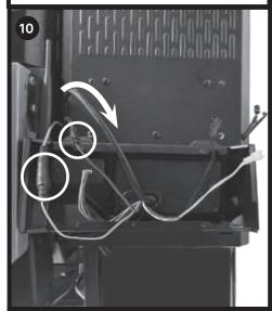
Disconnect 2 wire connections and feed the controller wire through the hopper pass through holes. Note, you will have to remove a zip tie from the inside of the hopper.
