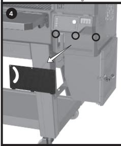
Remove 3 screws on the shutdown flap hopper shroud. Remove the shroud.
