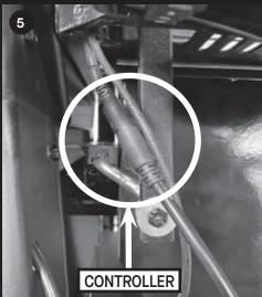
Remove the controller connections.
