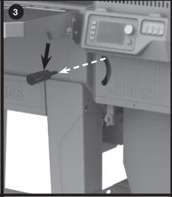
Remove 1 screw on the shutdown flap handle. Unscrew the shutdown slide handle.
