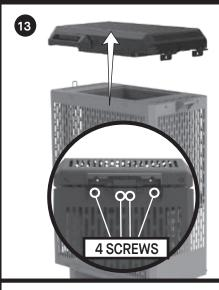
Remove the hopper lid from the shroud (4 Screws) Keep the hinge attached to the lid, you will reuse this.
