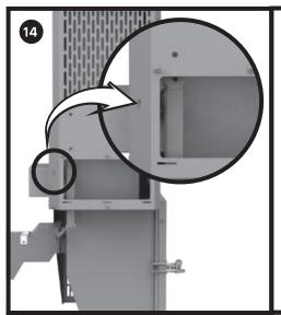
Disconnect the spring from the top shutdown flap assembly. Note: it is recommended to use a pair of needle nose pliars to accomplish this
