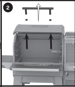
Remove lid handle and (2) bezels (2 screws). Save for reuse.
