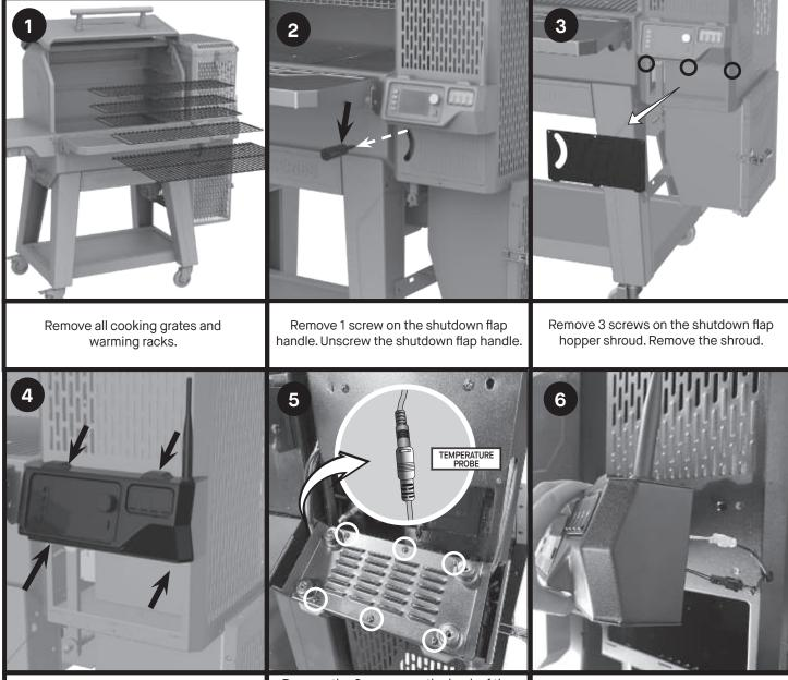
Remove the 4 thumb screws from the back of the controller. Remove the controller
